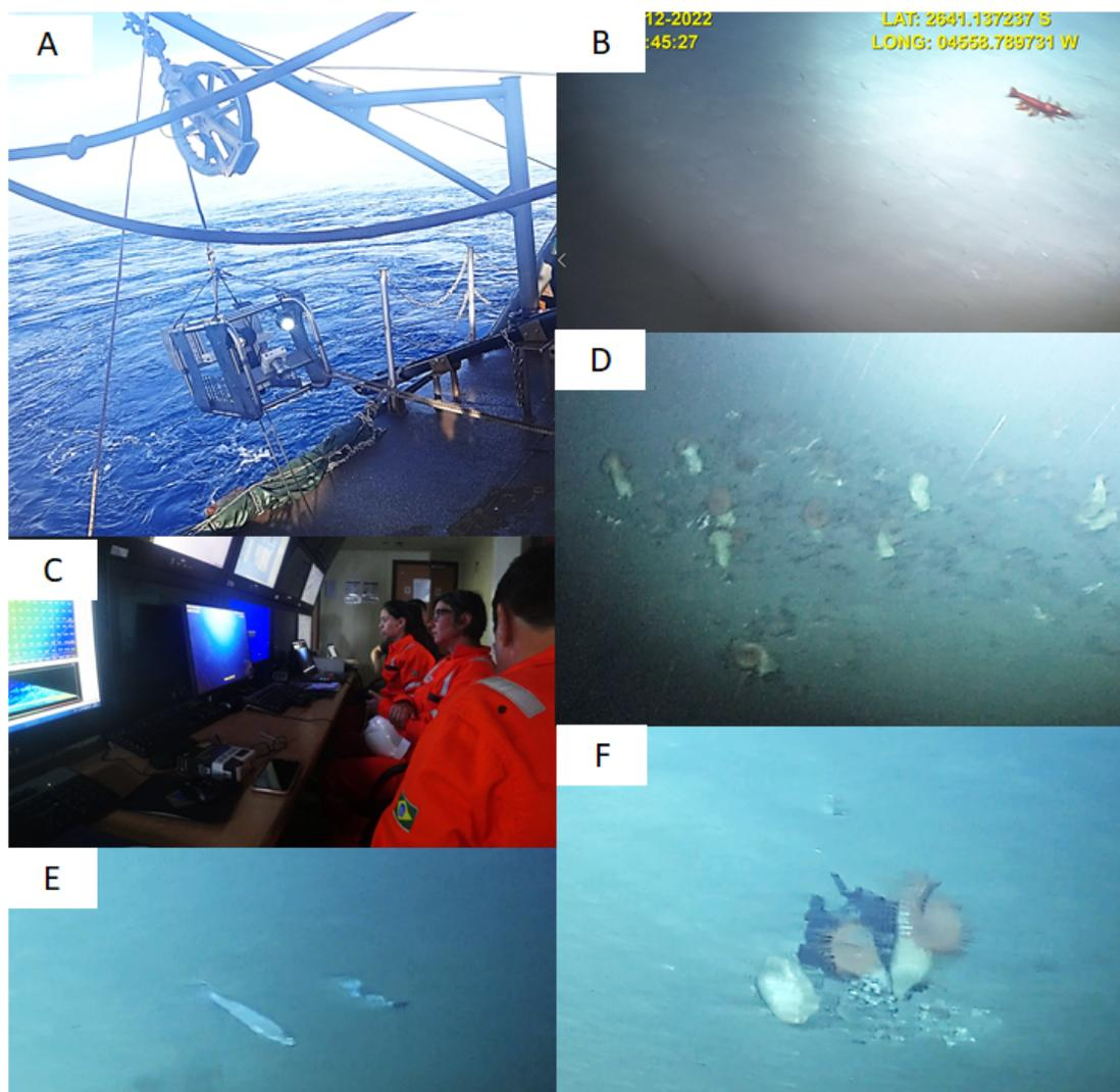
**Figure 4.** Towcam system operated during the iAtlantic\_BR10-Petrobras cruise. A) stern deployment of the towcam 'fish' C) towcam control center in the RV Vital de Oliveira dry lab; B, D, E, F) seafloor images produced by the towcam system on ~800 m deep areas. B) deep sea shrimp Family Aristeidae; D and F) anemones and sponges; E) fish Order Ophidiiformes.
