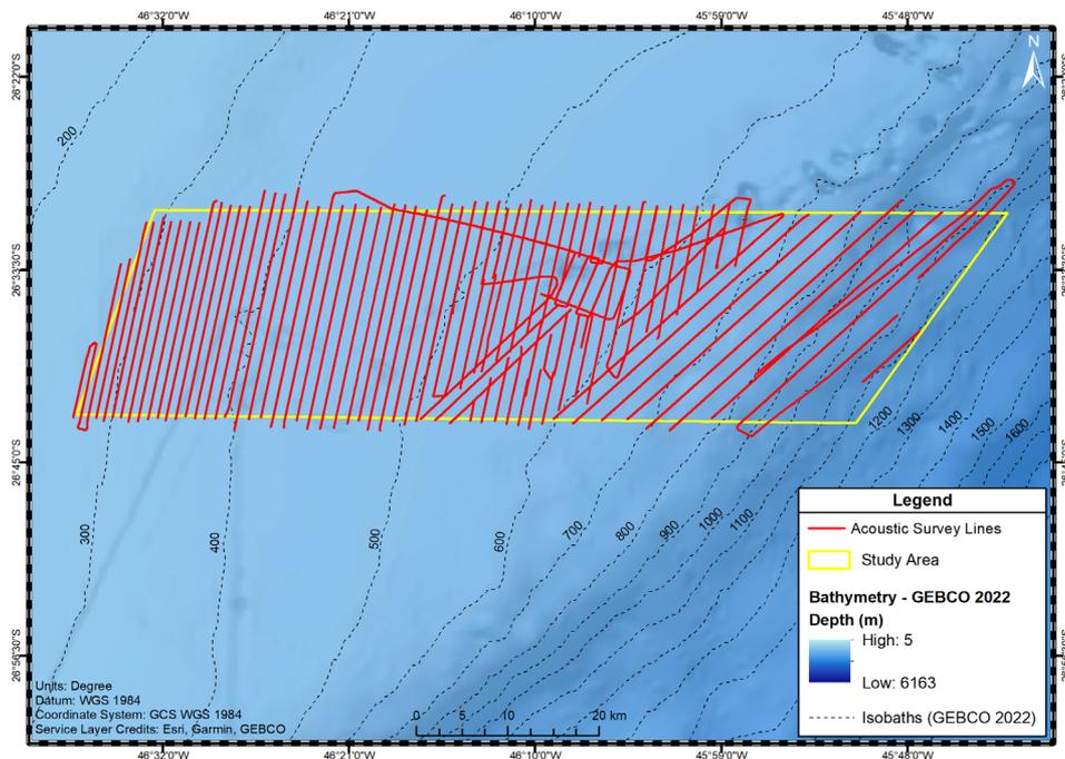
**Figure 2.** Multibeam echosounder and sub-bottom profiler track lines of the iAtlantic\_BR10-Petrobras cruise.
