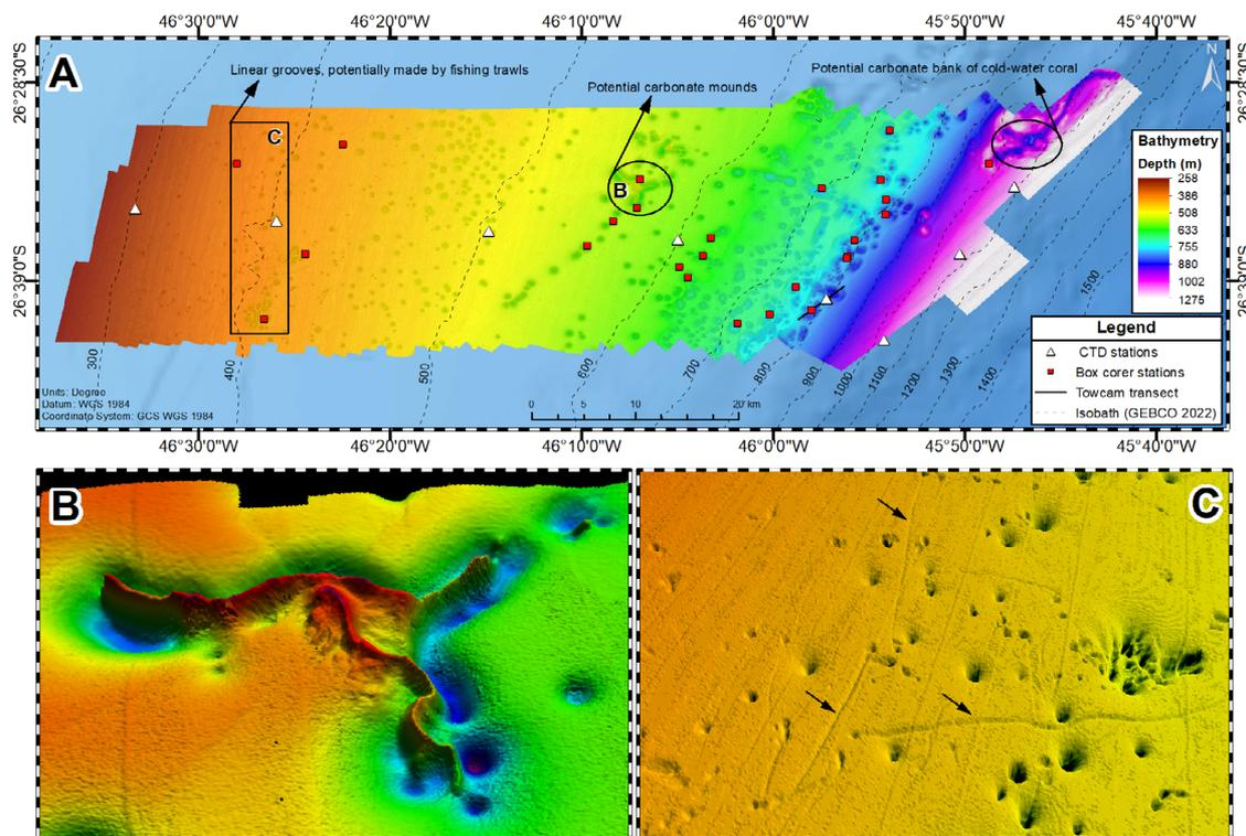
**Figure 3.** Bathymetric map of the study area produced during the iAtlantic\_BR10-Petrobras expedition (A). Red squares indicate stations with box corer deployments. White triangles indicate stations with CTD casts. A black line indicates the towcam transect position. B) 3-D view of the seafloor showing a large geological feature identified as potential carbonate mounds (Figure 1) and pockmarks. C) 3-D view of seafloor showing linear grooves (~400 m-deep) possibly made by fishing trawls.
